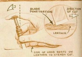
HOLD KNIFE AS SHOWN ABOVE. TIP FORWARD SO POINT OF BLADE CAN PENETRATE THE LEATHER. DOWNWARD PRESSURE WITH YOKE FINGER IS REQUIRED, TO CUT CURVES, ROTATE BARREL IN THUMB AND FINGERS. PRACTICE THE CUTS SHOWN BELOW, ON SCRAPS. PRACTICE, PRACTICE.
